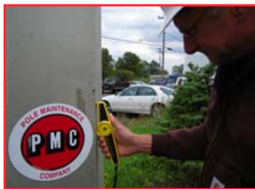
Zinc or Coating Thickness Test
