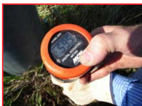
Corrosion Voltage Potential
